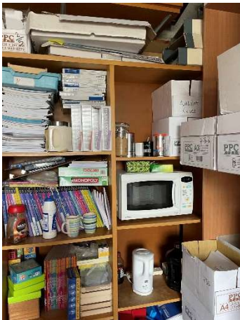
Figure 05 An example of a microwave in a temporary space that must be checked to ensure correct air flow around it
